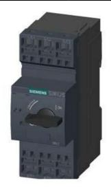
CIRCUIT-BREAKER SZ S0, FOR MOTOR PROTECTION, CLASS 10, A-REL. 9..12.5A, N-REL. 163A, SPRING-L. CONNECTION, STANDARD SW. CAPACITY
