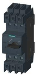
CIRCUIT-BREAKER SZ S00, FOR PLANT PROTECTION, WITH APPROBATION CIRCUIT-BREAKER UL 489. CSA C22.2 NO.5-02. A-RELEASE 5 A, N-RELEASE 65 A, SCREW CONNECTION, STANDARD SW. CAPACITY
