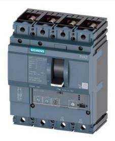
CIRCUIT BREAKER 3VA2 IEC FRAME 160 BREAKING CAPACITY CLASS C ICU=110KA @ 415 V 4POLE, LINE PROTECTION ETU320, LI, IN=100A OVERLOAD PROTECTION IR=40A ...100A SHORT CIRCUIT PROTECTION II=12 X IN NEUTRAL PROTECTION ADJUSTABLE(OFF,50%,100%) BUSBAR CONNECTION
