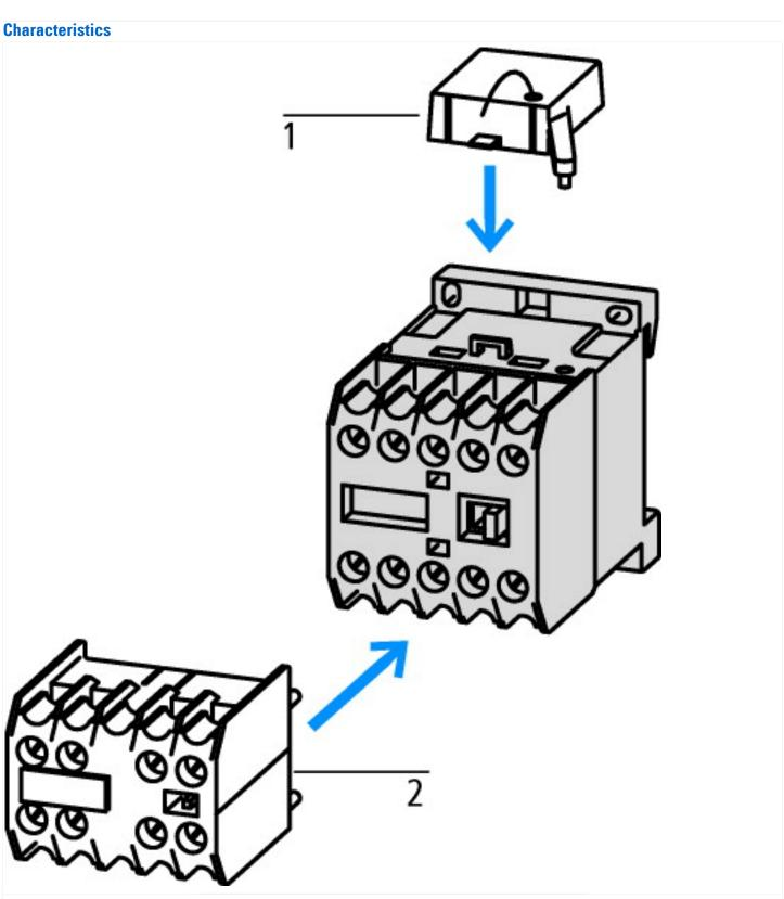
1: Suppressor 2: Auxiliary contact module
