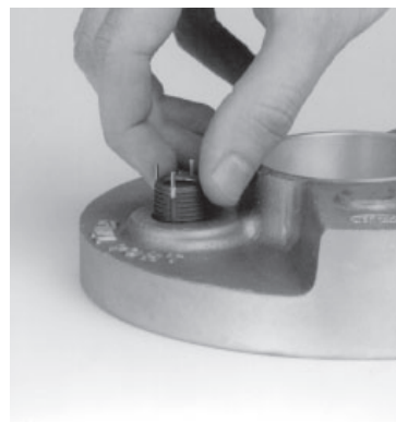
3. Screw the Clav-Sert insert into the housing
