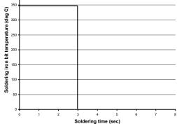
The soldering iron tip temperature should be set at 350°C (+10°C maximum) with the soldering duration not to exceed more than 3 seconds.
