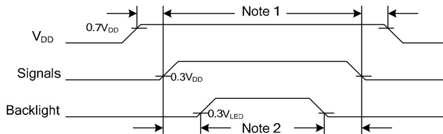
Note 1: In order to avoid any damages,  $V_{DD}$  has to be applied before all other signals. The opposite is true for power Off where  $V_{DD}$  has to be remained on until all other signals have been switch off. The recommended time period is 1 second. Hot plugging might cause display damage due to incorrect power sequence, please pay attention on interface connecting before power on.
