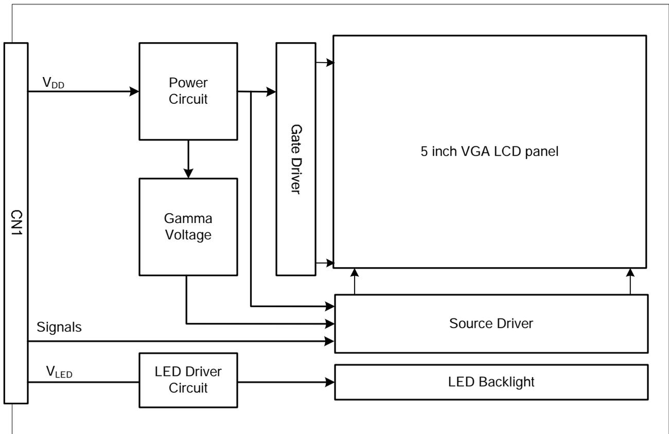
Note 1: Signals are DCLK, DE, and RGB data bus.
