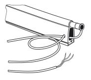
Slide the emitter and receiver into the upper chamber.
