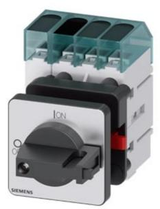
Switch disconnector 3LD3, main switch 3-polig + N, lu 25A operational switch at AC-23 A at 400 V 9,0 kW front mounted Base mounting with center-hole 22,5 mm knob-operated mechanism black  $48 \times 48$  mm
