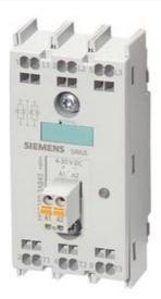
SOLID STATE RELAY 3-PHASE 3RF2 30 A 40 DEG. C 48-600 V / 4-30 V DC 2PH.-CONTROLLED SPRING-TYPE TERMINALS BLOCKING VOLTAGE 1200 V
