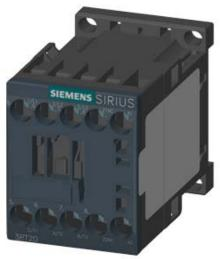
CONTACTOR, AC-3, 3KW/400V, 1NC, AC110V, 50/60 HZ, 3-POLE, SZ S00 SCREW TERMINAL
