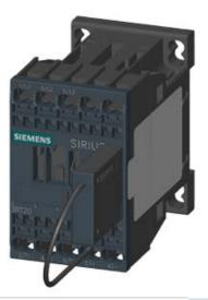
CONT. F. RAILW. A., AC-3, 5.5KW 5.5KW/400V,DC125V,0.7...1.25\*US W.SUPPRESSORDIODE INTEGRATED, 3-POLE, SZ. S00, SPRING-LOADED TERMINAL
