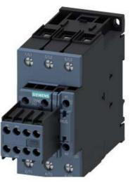
CONTACTOR,AC3:37KW/400V, 2NO+2NC, 20-33V AC/DC, WITH VARISTOR, 3-POLE, SIZE S2, SCREW TERMINAL
