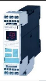
DIGITAL MONITORING RELAY CURRENT MONITORING, 22.5MM FROM 2 TO 500MA AC/DC OVERSHOOT AND UNDERSHOOT AC/DC 24 TO 240V DC AND AC 50 TO 60 HZ STARTUP AND INTERF. PEAK DELAY 0.1 TO 20S HYSTERESIS 0.1 TO 250MA 1 CHANGEOVER CONTACT W. OR W/O ERROR LOG SPRING-LOADED TYPE
