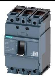
CIRCUIT BREAKER 3VA1 IEC FRAME 160 BREAKING CAPACITY CLASS N ICU=25KA @ 415 V 3-POLE, LINE PROTECTION TM210, FTFM, IN=100A OVERLOAD PROTECTION IR=100A FIXED SHORT CIRCUIT PROTECTION II=10 X IN BUSBAR CONNECTION
