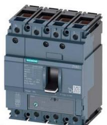
CIRCUIT BREAKER 3VA1 IEC FRAME 160 BREAKING CAPACITY CLASS H ICU=70KA @ 415 V 4-POLE, LINE PROTECTION TM220, ATFM, IN=16A OVERLOAD PROTECTION IR=11,2A ... 16A SHORT CIRCUIT PROTECTION II=10 X IN NEUTRAL PROTECTION 100% CABLE CONNECTION
