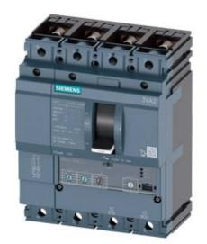
CIRCUIT BREAKER 3VA2 IEC FRAME 100 BREAKING CAPACITY CLASS H ICU=85KA @ 415 V 4POLE, LINE PROTECTION ETU320, LI, IN=40A OVERLOAD PROTECTION IR=16A ...40A SHORT CIRCUIT PROTECTION II=12 X IN NEUTRAL PROTECTION ADJUSTABLE(OFF,100%) BUSBAR CONNECTION
