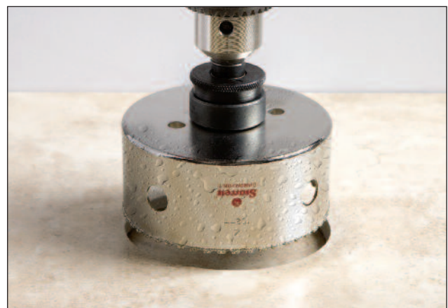
Diamond Grit Hole Saw Application.
