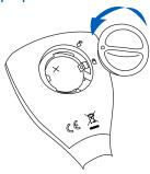
To change the CR2032 Li-ion battery, turn the battery cover located on the back of the meter counterclockwise to unlock. Remove cover and replace with + side facing up.
