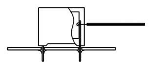
Temperature monitored inside the capacitor.
