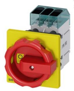
Switch disconnector 3LD3, main switch 3-polig, Iu 40A operational switch at AC-23 A at 400 V 15,0 kW front mounted Base mounting with center-hole 22,5 mm knob-operated mechanism red/yellow 66 x66 mm
