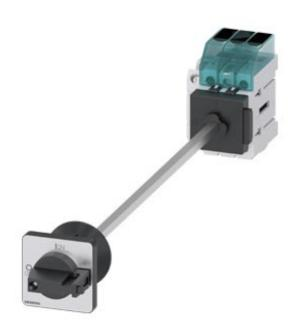
Switch disconnector 3LD3, main switch 3-polig, lu 63A operational switch at AC-23 A at 400 V 22,0 kW floor mounting Base mounting with door coupling center-hole 22,5 mm knob-operated mechanism black 48 x 48 mm with auxiliary 1NO+1NC
