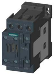
CONTACTOR, AC-3, 18.5KW/400V, 1NO+1NC, DC 48V, 3-POLE, SZ SO SCREW TERMINAL
