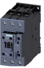
CONTACTOR,AC3:18.5KW/400V, 1NC+1NO,200VAC50HZ/200.220V60HZ 3-POLE, SIZE S2, SCREW TERMINAL
