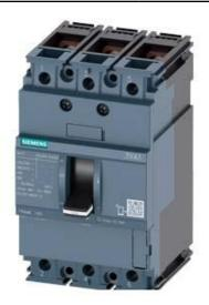
CIRCUIT BREAKER 3VA1 IEC FRAME 160 BREAKING CAPACITY CLASS S ICU=36KA @ 415 V 3-POLE, LINE PROTECTION TM210, FTFM, IN=100A OVERLOAD PROTECTION IR=100A FIXED SHORT CIRCUIT PROTECTION II=10 X IN BUSBAR CONNECTION
