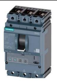
CIRCUIT BREAKER 3VA2 IEC FRAME 100 BREAKING CAPACITY CLASS L ICU=150KA @ 415 V 3POLE, LINE PROTECTION ETU350, LSI, IN=63A OVERLOAD PROTECTION IR=25A ...63A SHORT CIRCUIT PROTECTION ISD=1,5... 10 X IR, II=12 X IN BUSBAR CONNECTION
