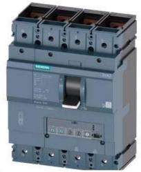
CIRCUIT BREAKER 3VA2 IEC FRAME 630 BREAKING CAPACITY CLASS M ICU=55KA @ 415 V 4-POLE, LINE PROTECTION ETU330, LIG, IN=400A OVERLOAD PROTECTION IR=160A ...400A SHORT CIRCUIT PROTECTION II=1,5...12 X IN NEUTRAL PROTECTION ADJUSTABLE(OFF,50%,100%) GROUND-FAULT-PROTECTION IG=0,2... 1 X IN, TG=0,1/0,3MS BUSBAR CONNECTION
