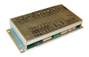
The Thermal Management System (TMS) is a flexible and fully configurable controller that can be used with EC/DC four wire speed controlled fans. Each fan can be individually speed controlled against one of the two temperature sensor inputs. The controller has four Solid State Relays (SSR's) that can be individually configured to give an alarm output against speed or temperature.
