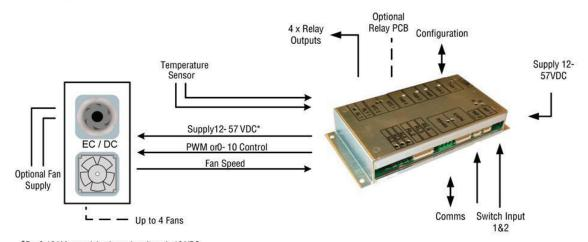
\*For 0-10 V fans, minimal supply voltage is 16 VDC For open collector fans, minimum supply is 12 VDC
