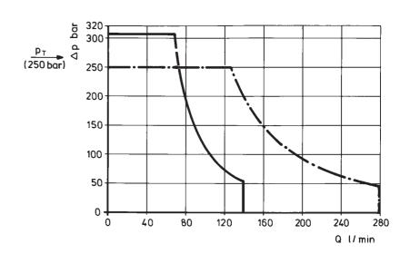
$\begin{array}{l} \textbf{Doubled flow rate} \\ p_{\text{max}} = 250 \text{ bar} \end{array}$
