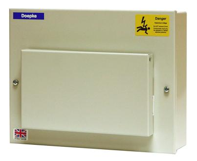
**DME IP2X** metal enclosures are suitable for use in domestic and similar installations covered by Amendment 3 regulations. They are manufactured from 1mm CR4 cold reduced mild steel, phosphate pre-treated and powder coated to RAL 9001. Cable knockouts are provided at 25mm and 20 mm top and bottom with large rear knockouts. The hinged metal flap has a magnetic fastener. Neutral and earth terminals are fitted along with din rail which accepts any of our modular devices.
