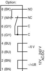
The relay-functions "NC" and "NO" bear on the switching mode "Dark-ON". This complies to the default setting of the light/dark
