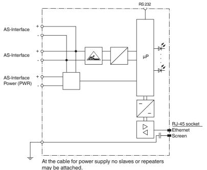
At the cable for AS-Interface circuit no power supplies or further masters may be attached.
