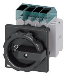
Switch disconnector 3LD3, main switch 3-polig + N, lu 32A operational switch at AC-23 A at 400 V 11,5 kW front mounted Base mounting with center-hole 22,5 mm rotary operationg mechanism black 66 x66 mm with auxiliary 1NO+1NC
