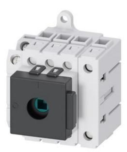
Switch disconnector 3LD3, main switch 3-polig + N, lu 40A operational switch at AC-23 A at 400 V 15,0 kW Distribution board mounting Base mounting with knob-operated mechanism with auxiliary 1NO+1NC
