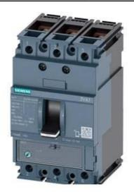
CIRCUIT BREAKER 3VA1 IEC FRAME 160 BREAKING CAPACITY CLASS H ICU=70KA @ 415 V 3-POLE, LINE PROTECTION TM220, ATFM, IN=20A OVERLOAD PROTECTION IR=14A ...20A SHORT CIRCUIT PROTECTION II=10 X IN BUSBAR CONNECTION
