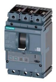
CIRCUIT BREAKER 3VA2 IEC FRAME 100 BREAKING CAPACITY CLASS M ICU=55KA @ 415 V 3POLE, LINE PROTECTION ETU350, LSI, IN=40A OVERLOAD PROTECTION IR=16A ...40A SHORT CIRCUIT PROTECTION ISD=1,5... 10 X IR, II=12 X IN BUSBAR CONNECTION
