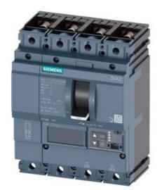
CIRCUIT BREAKER 3VA2 IEC FRAME 160 BREAKING CAPACITY CLASS H ICU=85KA @ 415 V 4POLE, LINE PROTECTION ETU550, LSI, IN=100A OVERLOAD PROTECTION IR=40A ...100A SHORT CIRCUIT PROTECTION ISD=0,6..10X IN, II=1,5..12X IN NEUTRAL PROTECTION ADJUSTABLE (OFF, UPTO 160%) BUSBAR CONNECTION
