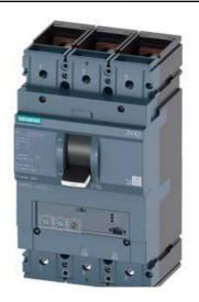
CIRCUIT BREAKER 3VA2 IEC FRAME 400 BREAKING CAPACITY CLASS C ICU=110KA @ 415 V 3-POLE, LINE PROTECTION ETU320, LI, IN=250A OVERLOAD PROTECTION IR=100A ...250A SHORT CIRCUIT PROTECTION II=12 X IN BUSBAR CONNECTION
