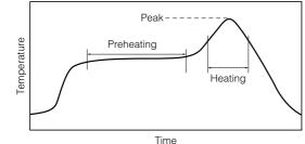
Recommended soldering conditions for flow
