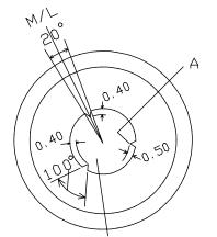
INTERCHANGABLE CORES SEE SHAFT LOCATION DRWG CL170810P2 FOR OTHER SHAFT HOLE DETAILS
