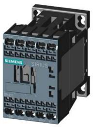
COUPLING CONTACTOR RELAY RAIL, 2NO+2NC, DC 110V, 0.7..1.25\*US, VARISTOR INTEGRATED, SZ S00, SPRING-LOADED TERMINAL FOR STANDING MOUNTING POSITION
