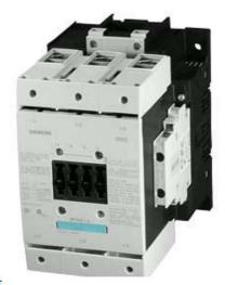
CONTACTOR, 55KW/400V/AC-3, AC(40...60HZ)/DC OPERATION UC 440...480V AUX. CONTACTS 2NO+2NC, 3-POLE, SIZE S6 WITH BOX TERMINALS CONVENTIONAL OPERATING MECHAN. SCREW TERMINAL
