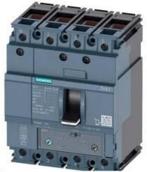
CIRCUIT BREAKER 3VA1 IEC FRAME 160 BREAKING CAPACITY CLASS S ICU=36KA @ 415 V 4-POLE, LINE PROTECTION TM240, ATAM, IN=160A OVERLOAD PROTECTION IR=112A ...160A SHORT CIRCUIT PROTECTION II=5...10 X IN NEUTRAL UNPROTECTED CABLE CONNECTION
