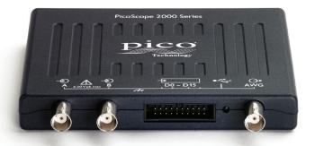
2+16-channel mixed-signal oscilloscope (MSO)
