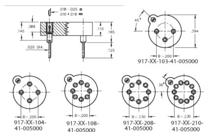
**Description:** Transistor TO Socket Through-Hole Mount Accepts .015"- .025" (0,38 - 0,635 mm) dia leads Through Hole
