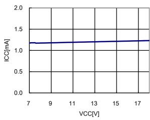
Figure 6. Operating current (ICC) vs VCC
