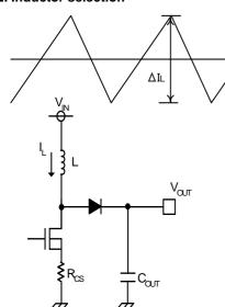
The inductor value affects the input ripple current. The equality in the section 3.5.1 is as following.
