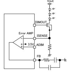
Figure 14. ISENSE pin circuit
