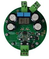
The EVAL\_AUDAMP25 MA5332 evaluation board is a twochannel, 200 W/ch (4  $\Omega$  at ±36.5 V; with heatsink) halfbridge class D audio power amplifier for Hi-Fi audio systems. This evaluation board demonstrates how to use MA5332 IC, implement protection circuits, and design an optimum PCB layout using Infineon integrated Class D IC. This reference design does not require additional heatsink or fan cooling for normal operation (one-eighth of continuous rated power).
