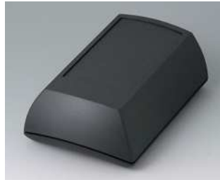
B7015209 ERGO-CASE M, hoch ABS (UL 94 HB) schwarz RAL 9005 150x100x55mm IP 54 opt.
