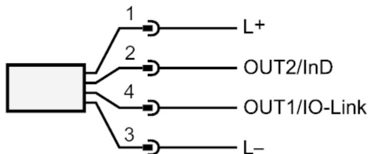
OUT1/IO-Link: switching output volumetric flow quantity monitoring
