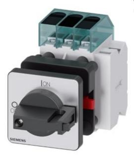
Switch disconnector 3LD3, main switch 3-polig, Iu 40A operational switch at AC-23 A at 400 V 15,0 kW front mounted Base mounting with center-hole 22,5 mm knob-operated mechanism black 48 x 48 mm with auxiliary 1NO+1NC
